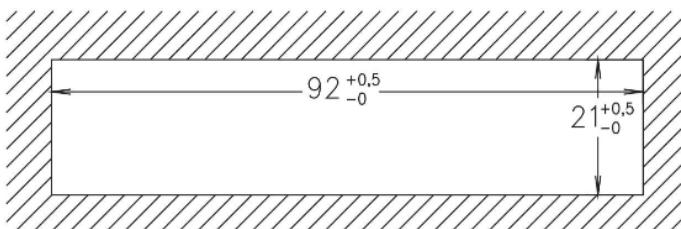
Wall thickness max. 5mm
